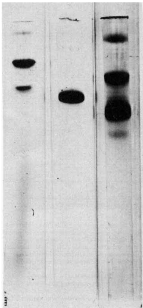
Figure 4 —Comparison of electrophoretic patterns of anion-exchange gel-chromatographic gel Fraction G2, peak B (Gel A); anion-exchange gel-chromatographic gel Fraction G3, peak B (Gel B); and chromatographic gel peak C (Gel C) on 12% polyacrylamide gels.
